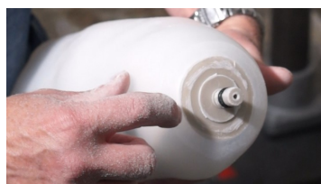
Sand flexible inner down so anchor is almost 100% exposed
