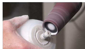
Sand flexible inner down so anchor is almost 100% exposed
