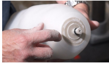
Sand flexible inner down so anchor is almost 100% exposed
