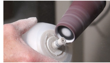
Sand flexible inner down so anchor is almost 100% exposed
