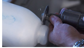
Cut tooling free with cast saw, knife or utility knife.
