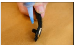
6 Use Loctite 242 on 6x14 screw.
