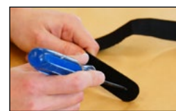
4 Use a hot awl or punch to make a hole for 6x14 screw. Screw should fit through hole easily.
