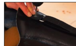
9 Use lanyard strap to attach chafe in proper location.
