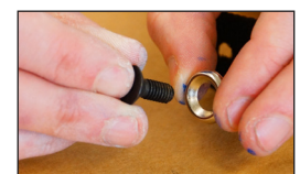
5 Put 6x14 screw and liner washer through hole in the lanyard strap.
