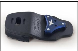
**1** The pyramid adjustment slot on top of keel gives the pyramid 14 mm of slide from side to side. This makes it possible for the foot to be adjusted for a right or left pedal.
