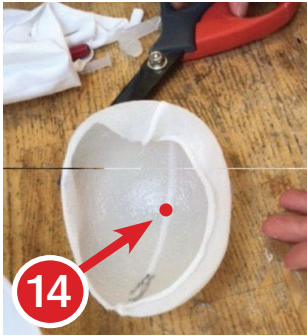
14) Punch a 1/2" CENTER HOLE in the pad to allow vacuum to pass through the silicone.
