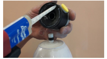
9. Pull a PVA bag over the anchor and cast. Glue your lock to anchor and start laminating.
