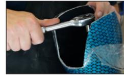
**49** Use the Threaded Bolt and 3/4" socket wrench to push the dummy out.
