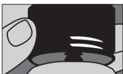
**ii** Install pin on liner. Engage lock to check for play between lock and liner.
