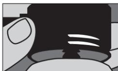
**viii** After installing pin spacers, re-engage lock to be sure there is no play.
