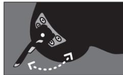
**60** Lever is shown open (UNLOCKED). When lever is flush, lock is engaged (CLOSED).
