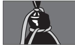
**43** String can be tied between fabrication plug and top of lock to ensure seal (see Caution #6).
