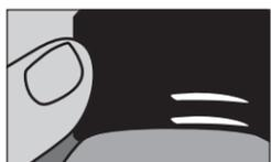
**iv** Reengage lock to check for play. Repeat until lock seats completely.
