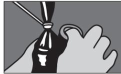
**42** Toward end of lamination, place tape over 5-hole plate to squeeze excess resin out of lamination.
