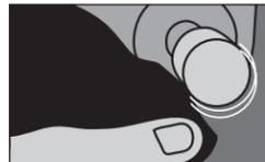
**48** Smooth out edges and bottom of socket. Remove socket in traditional fashion or with socket extractor.
