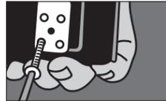
**46** Expose lamination dummy and remove screws.
