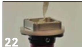
22 Check height measurement to ensure height is identical to test socket. Fill connector with glue.
