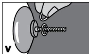
**v** Based on the gap size created by loosening pin, install appropriate number of pin spacers on the adaptor (see Attention A5).
