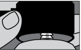
**H7** After installing pin spacers, re-engage lock to be sure there is no play.
