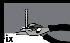
**ix** After hand tightening, tighten the brass adapter screw base against the liner a 1/4 turn more with a wrench or pliers.
