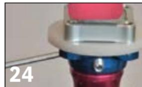
24 Remove mold (with lock and connector) from fixture.
