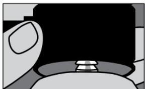
**H1** Install pin on liner. Engage lock to check for play between lock and liner.
