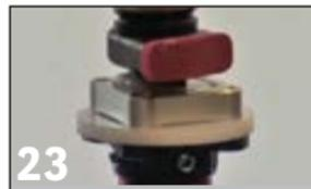
23 Lower mold and lock onto connector. Allow glue to set.
