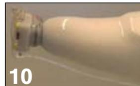
Vacuum form as usual. Press plastic into bottom of connector to reinforce it.
