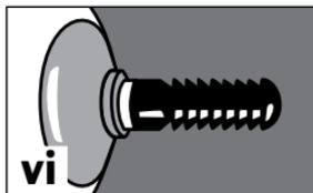
**vi** Replace pin on adaptor, making sure base fits snugly on pin spacers.
