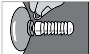
**H5** Based on the size of the gap created by loosening pin, install appropriate number of pin spacers on threaded end (see Attention A5).
