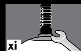
**xi** Now tighten pin assembly with pliers or vice grips to insure complete thread engagement of brass into liner and pin into brass. (See Attention A4, A5, A5)
