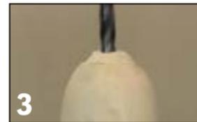
Drill a hole in the center of the flattened area to seat the anchor.
