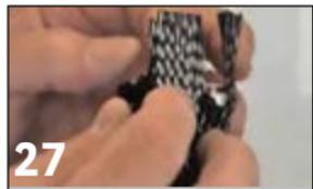
27 Fold carbon and other layup materials between connector posts. As layup material is added, ensure the connector posts remain exposed.
