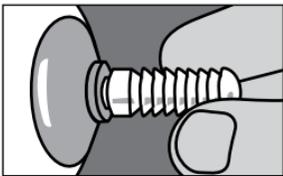
**H2** If there is play, loosen pin away from adapter screw and liner.
