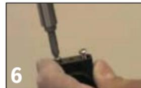
Install lamination tool using face plate screws.
