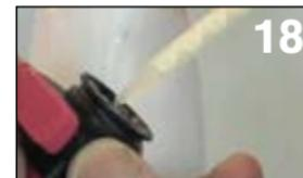
Apply a bead of glue to housing funnel and glue to anchor with lamination tool aligned with release button location mark.
