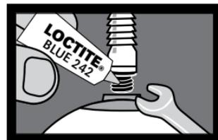
**H8** Apply Loctite® Blue 242 to threads of lock pin. Pin may need to be tightened with pliers or vice grips. (See Attention A5)
