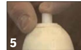
Place anchor screw into hole securing anchor to mold. Fill in any gap with plaster and smooth transition.
