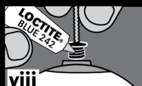
**viii** Apply Loctite® Blue 242 to threads of lock pin on adaptor screw threads. Screw into liner finger tight.
