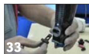
33 Slide lock plate into face plate and install spring.
