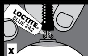
**x** Place needed number of pin spacers on adapter screw. Apply Loctite® Blue 242 to threads of lock pin adapter screw. Screw the 8 click pin finger tight.
