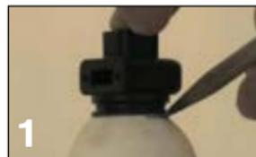
Remove Lock components from housing. Place housing on mold and trace its location.
