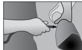
**S12** Once internal parts are removed blow out the chamber with compressed air.
