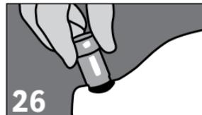
**26** Hand-tighten valve body with Coyote lock wrench or 13mm deep well socket.
