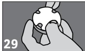
**29** Lube and install glue plate on Coyote Alignable Connector.
