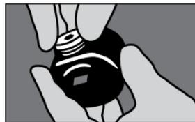
**12** Install Fabrication Plug in lock.
