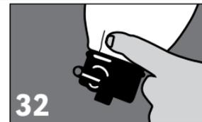
**32** Install lock on mold in desired location, mark release button location. (See Caution #1).
