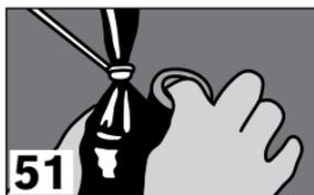
Toward end of lamination, tape can be placed over five hole plate to squeeze excess resin out of lamination.
