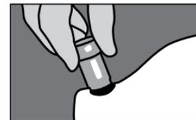
**S16** Hand-tighten the valve body very snug but not too tight with the lock wrench or 13mm deep well socket.
