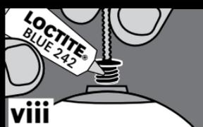
**viii** Apply Loctite® Blue 242 to threads of lock pin on adaptor screw 10 mm threads. Screw into liner finger tight.
