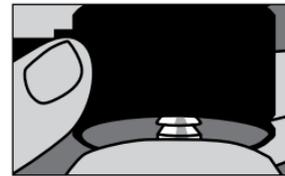
**H7** After installing pin spacers, re-engage lock to be sure there is no play.
