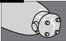
**18** For extra strength, fold excess seam on distal end of connector.
