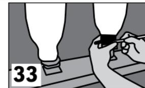
**33** Rest mold and lock on Alignable Connector. Place test socket next to mold and compare alignments.
