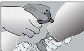
**S14** Clean the lock and socket with rubbing alcohol or mild soap and water and wipe it out with a towel.
