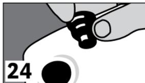
**24** Add third spring. Slide release button into valve body.
