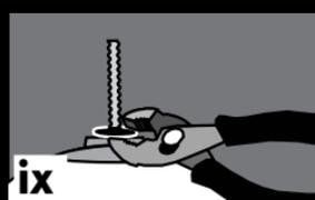
**ix** After hand tightening, tighten the brass adaptor screw base against the liner a 1/4 turn more with a wrench or pliers.
