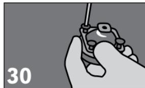
**30** Attach a pyramid to Coyote Alignable Connector.
