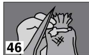
Pull first composite layer over mold. Cut top edges to fold around posts.
