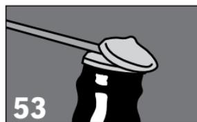
Expose edge and remove excess lamination.
