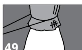
Tie second layer of composite under five hole plate and reflect down over mold.
