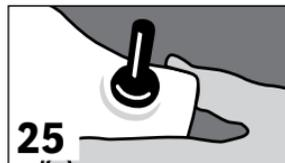
**25** Thread valve body into housing.
