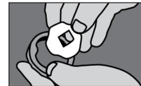
**14** Install insert of choice in Alignable Connector.
