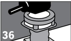
**36** Place mold and lock back into connector in desired location. Let set.
