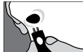
**22** Slide lock plate into lock, springs first. It slides easily ONLY one way. Verify orientation first. (See Caution #3)
