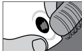
**21** Carefully smooth inside of hole to allow for easy assembly of lock.
