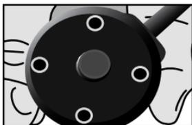
**G6** Place CD103PC Pin Cap on guide pin in hole. Use the guide pin to stop pin cap at correct depth in the hole.
