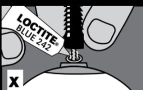
**x** Place needed number of pin spacers on adaptor screw. Apply Loctite® Blue 242 to threads of lock pin adaptor screw. Screw the 8 click pin finger tight.
