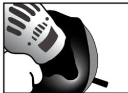
**G3** Using a 1/4" x 6" drill bit drill through the Guide Pin, lock and socket.
