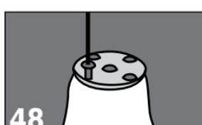
Lubricate screws and install five hole plate. (See Caution #C4)
