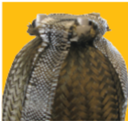
Criss crossing strips of carbon tape
